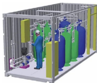
3D MODEL OF SELECTED TREATMENT SYSTEM.
